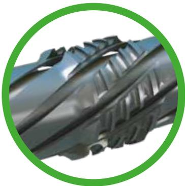
Each Eco-Max™ includes a single piece caged scraper element with 360° overlapping blades which ensure 100% casing wall coverage. The scraper features self-cleaning teeth to remove cement, perforation burrs, scale and other potentially damaging debris from the casing.
